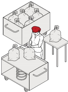
Figure 38 Self-adjusting base in laundry tubs reduces the need for bending, twisting and reaching during unloading.
